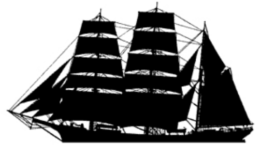
Typical rig of a barque --courtesy of the Maritime Museum of the Atlantic
