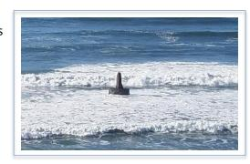
The pylon, originally sporting a 15-foot wooden octagon atop it, was reportedly a calibration target for the radar transmitters that had to be calibrated each time they were used. The octagon was a known distance from the transmitters, and the gunners used it to correlate readings, checking the radar's accuracy.
